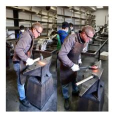
Blacksmith shapes and joins metal by heating it in a forge until it is soft and workable. He then hammer, bend and cut the metal into shape before it cools again. Blacksmith uses these skills to make items such as wrought-iron gates, railings, furniture and tools or artistic pieces.
